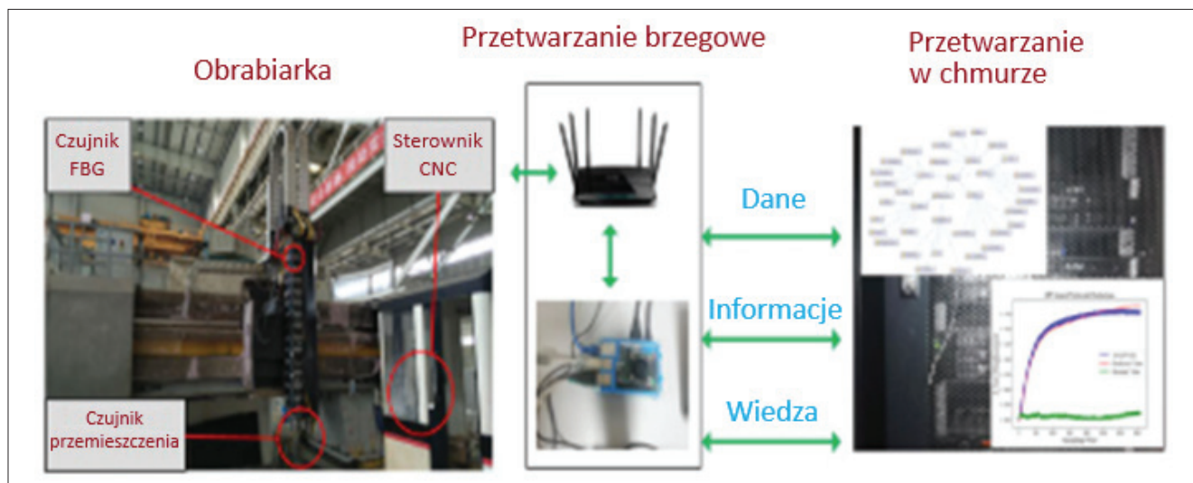
Fig. 2. Schematic representation of information collaboration in real IMT-ECC system (FBG – fiber bragg grating ) [2, 8]
