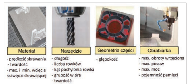
Fig. 6. Groups of input data using in so-called Technology Creator in IMachining program [2]
