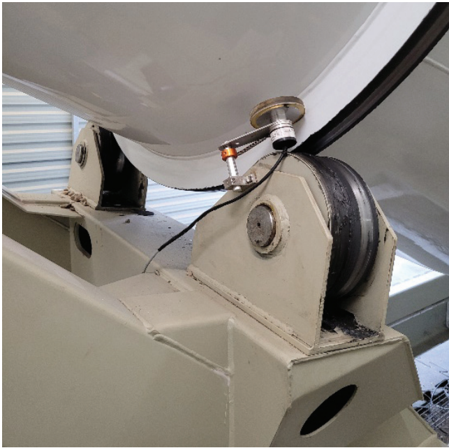
Fig. 3. Mixer drum rotational speed sensor
