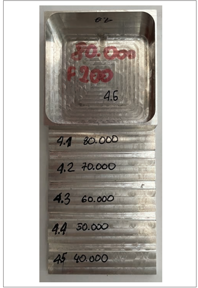
Fig. 2. A sample made of 7050 aluminum alloy, machined at cutting speeds v_c from 753.6 m/min (over 4.5) to 1507 m/min (over 4)
