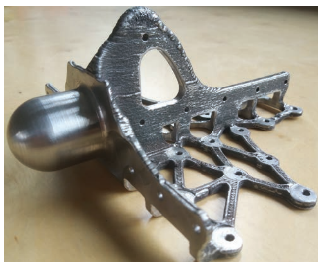
Fig. 7. Bracket made in AM technology of stainless steel material (SS410)
