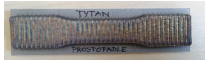
Fig. 10. Example of a test sample with layers applied perpendicularly
