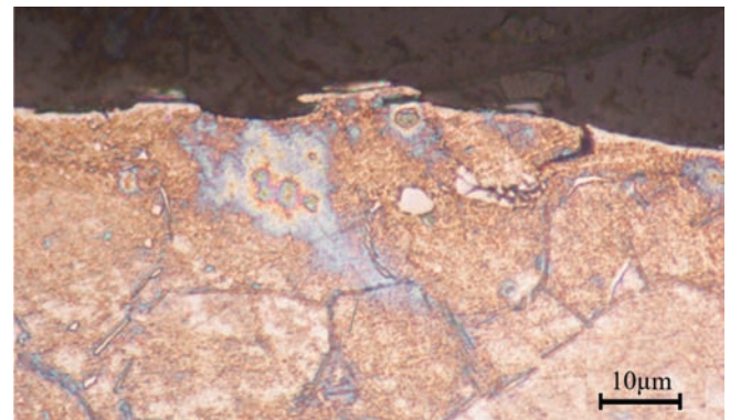
Fig. 6. Inconel 718 (20 HRC) microstructure after turning with WNMG 080408-TF IC3028; v_c = 40 m/min, f = 0.05 mm/rev, a_p = 0.20 mm, VB_C = 0.25 mm (visible microcracking)
