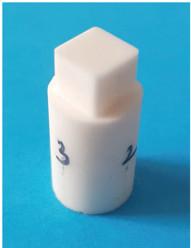
Fig. 7. Sample made with PCD05 tool ( v_c = 120 m/min, f_z = 0.05 mm/rev, a_p = 0.05 mm)
