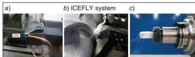
Fig. 10. Methods of delivering \text{LN}_2 to the cutting zone: a) internally and b) externally [18]; c) through the spindle for cryogenic MQL cooling [21]
