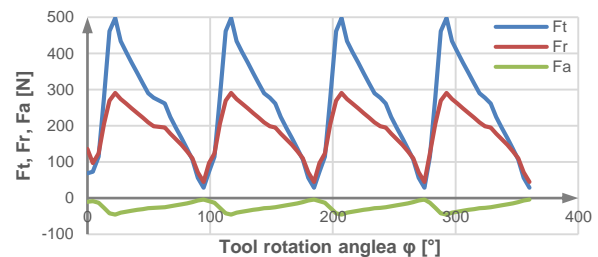
Fig. 6. Course of the cutting force components for the concave surface with curvature r_{k1} = -25 mm
