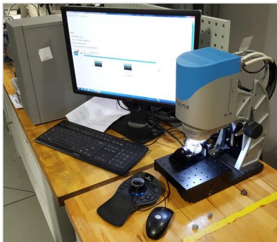
Fig. 3. Stand for measuring the radius of the rounding of cutting tool edges
