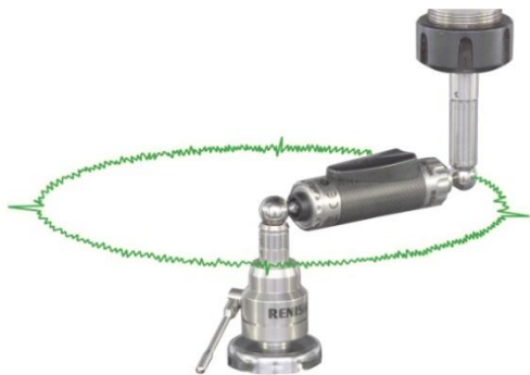
Fig. 2. System QC20-W ball bar [9]
