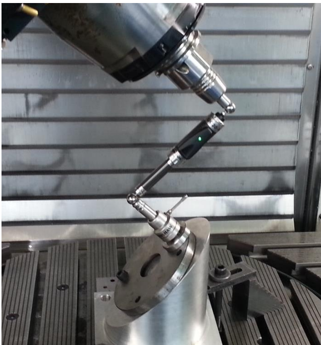
Fig. 3. Modified accuracy test of the machine tool [8]
