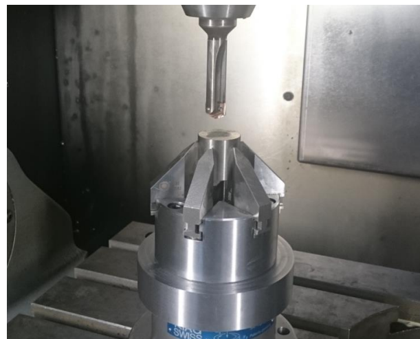
Fig. 1. Stand for measuring the moment and cutting force during drilling
