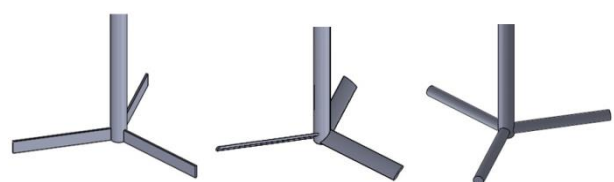
Fig. 2. Three types of agitator rotors (from the left): turbine blend, propeller agitator, agitator with roller blades
