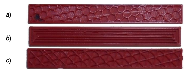
Fig. 2. Sample cross-section with a filling density of 30%. Fill type: a) hexagonal, b) concentric, c) triangular
