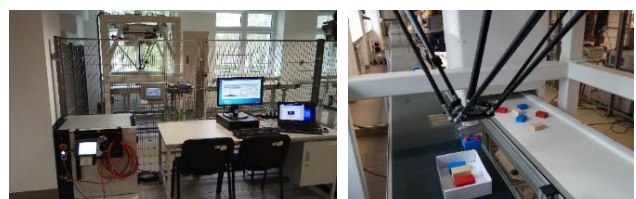
Fig. 3. Sorting station in Robotics Laboratory WAT with IRB360
