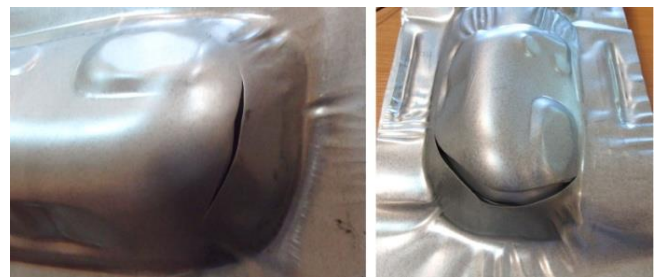
Fig. 1. Drawpiece with defects in the form of cracks and wrinkles
