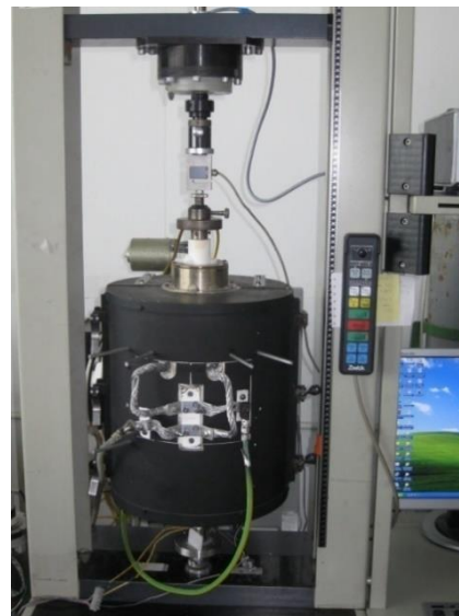
Fig. 4. Stand for measurements of fracture toughness at elevated temperature
