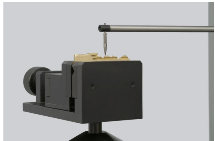
Fig. 3. Measurement of shape made with TOPO 02
