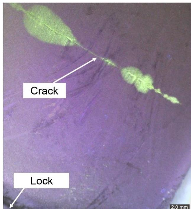
Fig. 8 The crack on the upper surface of the blade after a fatigue test
