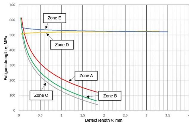
Fig. 6. Average fatigue strength of the blades depending on the length of defect - zone A-E
