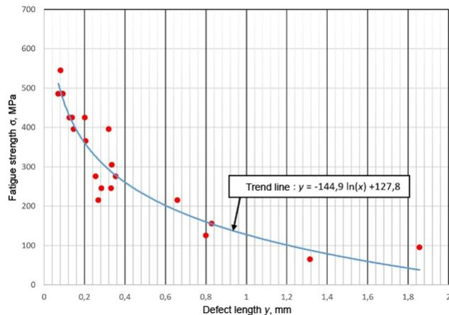
Fig. 5. Average fatigue strength of the blade as a function of defect length - zone C
