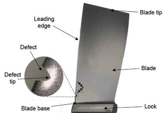
Fig. 3. Blade leading edge with defect in zone A; defect group - V
