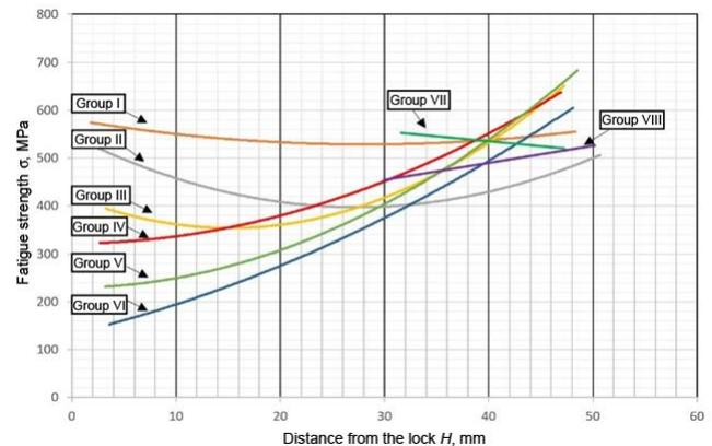
Fig. 7. Fatigue strength of the blades as a function of defect distance from the lock - defect group I-VIII
