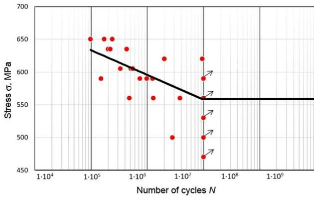
Fig. 4. Wöhler plot for the first stage vanes of an aircraft turbine compressor
