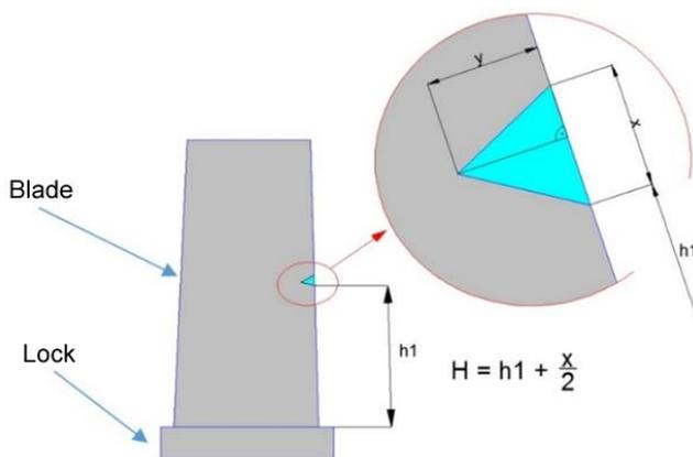
Fig. 1. Scheme of the compressor blade and defect measurement methodology
