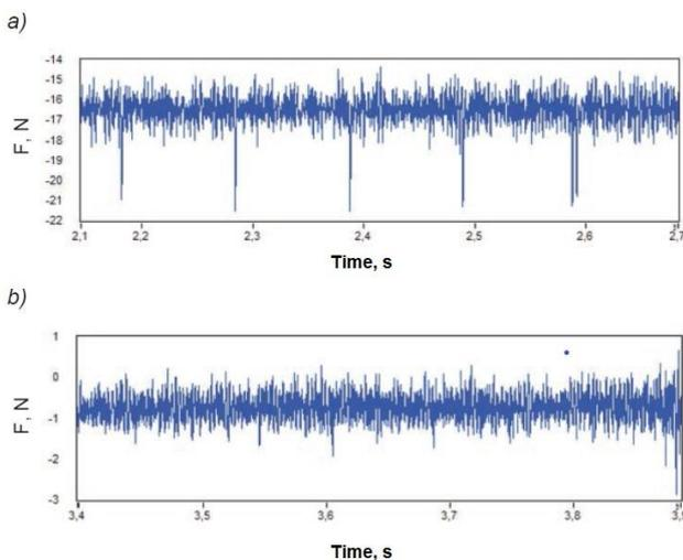
Fig. 1. Signal from the dynamometer: a) with disturbance and b) after removal of the disturbance
