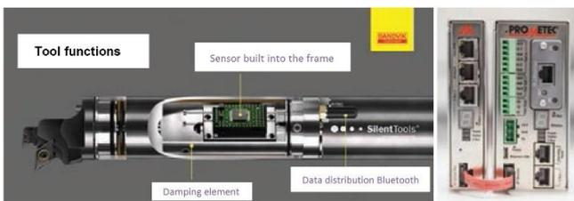
Fig. 2. Cutting process monitoring proposed by Sandvik and PROMETEC [13]
