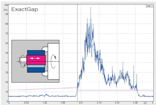
Fig. 5. Monitoring in the ExactControl system [16]
