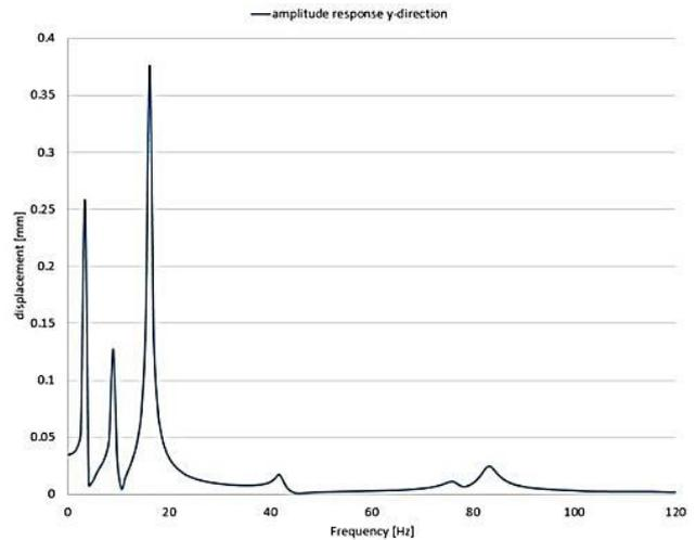
Fig. 3. Displacement value as a function of frequency for the HYDROPOL composite [14]
