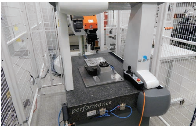
Fig. 1. The system consists of CNC electro discharge machine (Roboform 350 Sp GF Agie Charmilles) to manufacture the workpieces, 3R robot for loading workpieces and tools in and out of the machine and for using the identification cycles (Work Master robot) and CMM (DEA Global Performance, with measuring range 500 \times 700 \times 500 mm, resolution 1 \mu\text{m} )
